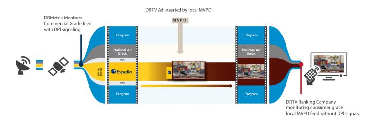
On the left side of the graphic, a cable network is shown sending its signal via satellite to a local MVPD. MVPD stands for "Multichannel video programming distributor" and describes companies that sell consumers access to cable programming. This includes companies that make television programming available via cable, satellite, fiber, or via internet.
